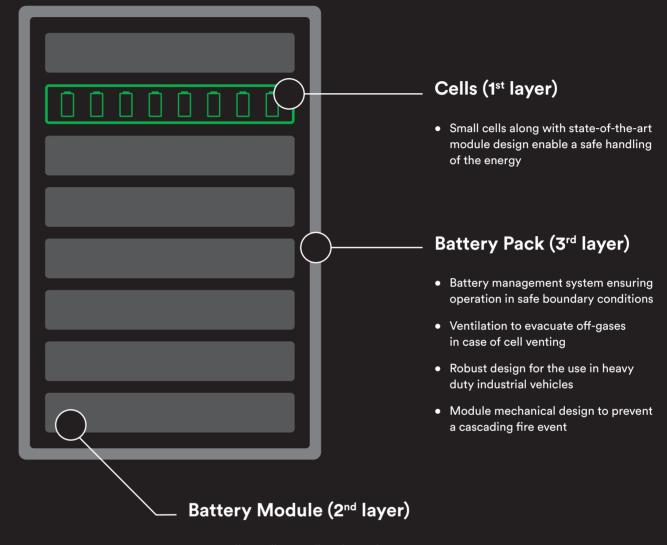
No cell to cell cascading thermal runaway with passing IEC 62619 propagation test
